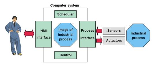
FIGURE 3. PROPOSED MODULAR DECOMPOSITION OF AN INDUSTRIAL CONTROL APPLICATION
