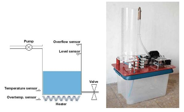
FIGURE 1-A DIAGRAM OF THE SCALE MODEL. 1-B REAL TANK DEVELOPED MODEL
