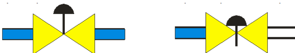
Figure 7: Representation of a digital valve in its two different states.
