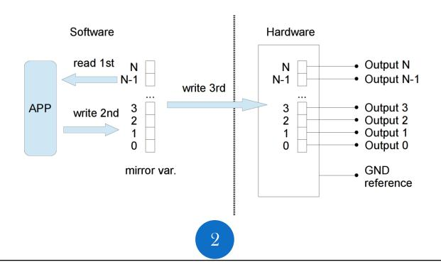
Figure 14: Diagram of the digital output subsystem.
