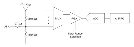
Figure 14: Blocks of the NI USB-6008 analog input section.
