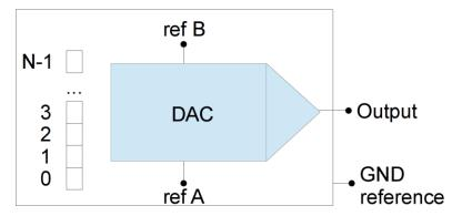
Figure 14: Blocks of a typical DAC converter.
