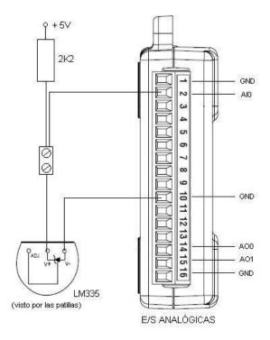
The + 5V supply can be obtained from the terminal block no. 31 of the digital I/O side of the DAQ card.
