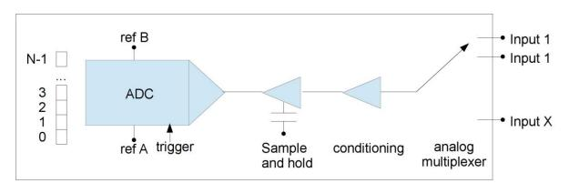
Figure 14: Blocks of a typical ADC conversion system.
