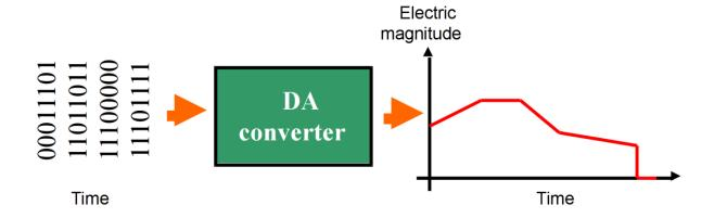
Figure 14: Representation of the digital to analog process conversion.
