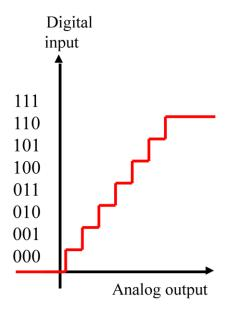
Figure 14: Stair effect of output of the DAC.
