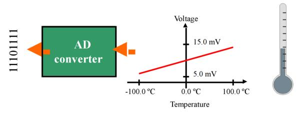
Figure 14: Representation of the analog to digital process conversion.
