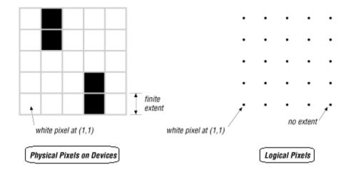
Figure 4: Physical pixels vs logial pixels
