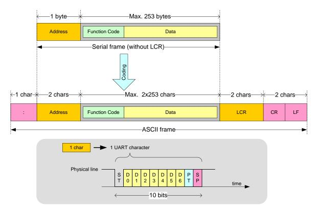
Figure 6 - ASCII transmission.
