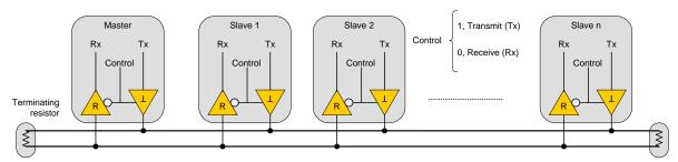
Figure 8 - RS-485 connections.
