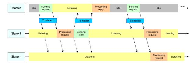
Figure 2 - Request/reply Exchange.
