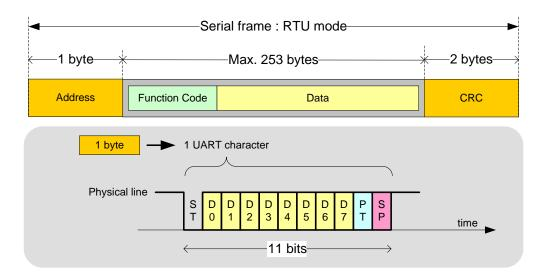
Figure 4 - RTU transmission.
