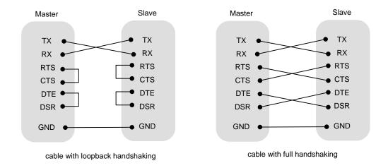
Figure 7 - RS-232 cable connections.
