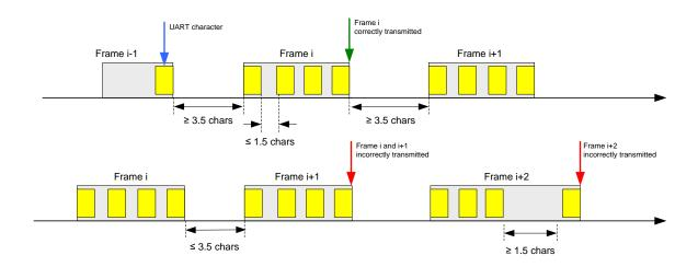
Figure 5 - RTU timing requirements.
