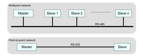
Figure 1 – Examples of Modbus serial networks.
