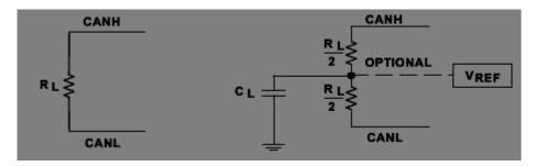
(figure from Microchip application note AN228 - Control Area Network Physical Layer Requirements)
